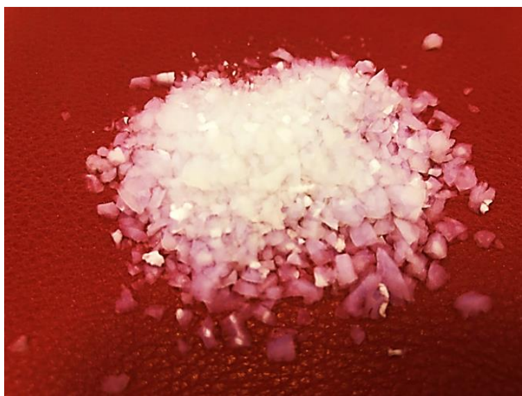
Figure 4.47. The produced silica aerogel material.
